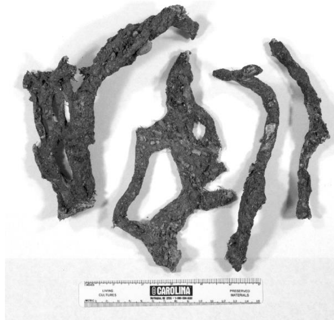
Figure 6 – Field-collected rhizomorphs of Meruliporia incrassata from an infested home in California. Note the root-like, woody appearance (Specimen courtesy Luis De La Cruz Wood Preservation Services, Pasadena, CA, USA; Photo courtesy of L. Yafetto).
